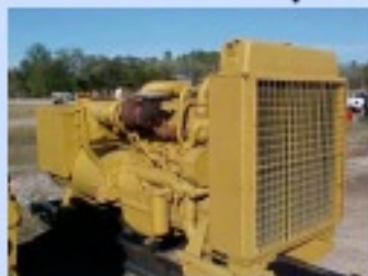
Cat 3406 Generator Set 175KW Prime/210 STDBY, 480 Volt Electric Start and Charging, WT and OP Safety Shutdown Load Tested.
