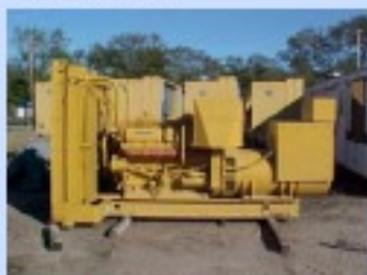
Cat 3412 DITTA Generator Sets , 545KW Prime/600 STDBY, 480 Volt Electric Start and Charging, EMCP Panel , Cat Rail Mounted. Low Hour Units, Load Tested.
