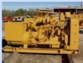
Cat 3306 Generator Set 135KW Prime, 480Volt Electric Start and Charging, WT and OP Safety Shutdowns, Skid Mounted. Load Tested.
