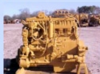
0 Hour and load tested 3406 Caterpillar power unit 375 hp 3 Available
