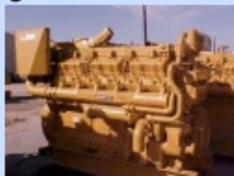
D398 "0" Hour Power Unit. 825 HP, Air Start, Premium Gauge Panel. WT, OP and OS Safety Shutdowns.
